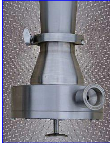
(6) Horns. S/N's: D45-51-169, D45-51-170, D45-51-171, D45-51-172, D45-51-173, and D45-51-174. Inlets/outlets: (1) 2-1/2 in. dia. NPT, (1) 4 in. dia. port. Overall dimensions: 10-1/2 in. dia. x 13 in. H.
