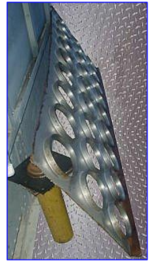
(12) Stainless Steel Plates with (27) 7-1/2 in. dia. ports per plate section. Overall dimensions: 86 in. L x 29-1/2 in. W x 2-1/4 in. H.
