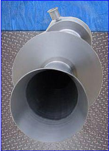
(6) Horns. S/N's: D45-51-169, D45-51-170, D45-51-171, D45-51-172, D45-51-173, and D45-51-174. Inlets/outlets: (1) 2-1/2 in. dia. NPT, (1) 4 in. dia. port. Overall dimensions: 10-1/2 in. dia. x 13 in. H.
