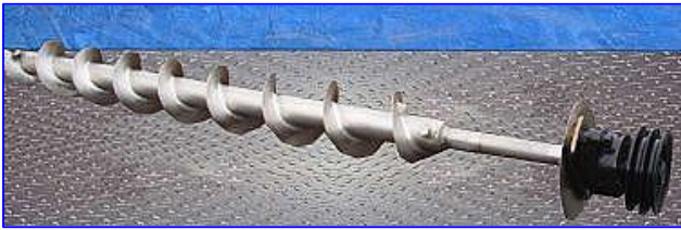
Stainless Steel Screw Auger. Auger dimensions: 6 in. dia. x 52 in. L. Pitch: 6 in. Shaft diameter: 1-1/8 in. Overall dimensions: 8 in. dia. x 72 in. L.
