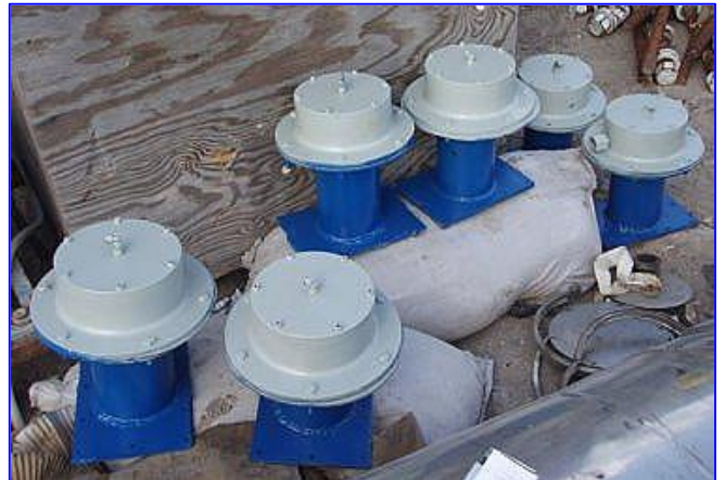
(6) Horns. S/N's: D45-51-169, D45-51-170, D45-51-171, D45-51-172, D45-51-173, and D45-51-174. Inlets/outlets: (1) 2-1/2 in. dia. NPT, (1) 4 in. dia. port. Overall dimensions: 10-1/2 in. dia. x 13 in. H.
