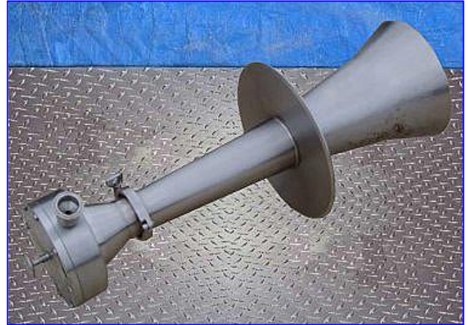
(6) Horns. S/N's: D45-51-169, D45-51-170, D45-51-171, D45-51-172, D45-51-173, and D45-51-174. Inlets/outlets: (1) 2-1/2 in. dia. NPT, (1) 4 in. dia. port. Overall dimensions: 10-1/2 in. dia. x 13 in. H.
