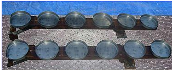
Stainless Steel Scaper Blade. Each blade section measures 46 in. L x 7 in. W. Shaft diameter: 2 in. Overall dimensions: 19 ft. 10 in. L x 9-1/2 in. W x 6 in. H.
